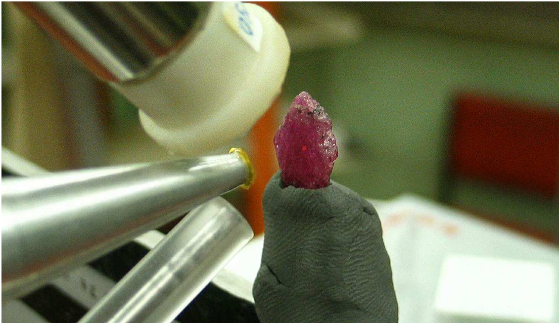
Figure 2. A mineralogical obsidian bombarded with external proton beam of 3 MeV energy for PIXE analysis. Due to ionoluminescence the analyzed spot is clearly seen in red on this particular sample.
