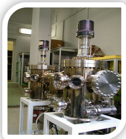
Figure 4. (a)- The experimental setup for generation of high homogeneity Rubidium plasma, (b)- Ionization efficiency of Rb atoms as a function of laser pulse energy in logarithmic scale.
