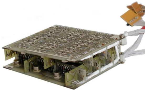
Figure 2. Power switch module developed by our team which switched the power for five sensors of Rosetta Plasma Consortium instrument.
