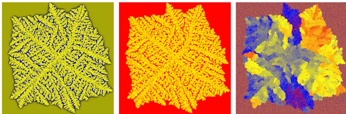
Figure 2. Interaction of a growing dendrite with foreign particles represented by 'orientation pinning centers' in the HMP model. From left to right: composition, phase-field, and orientation maps.
