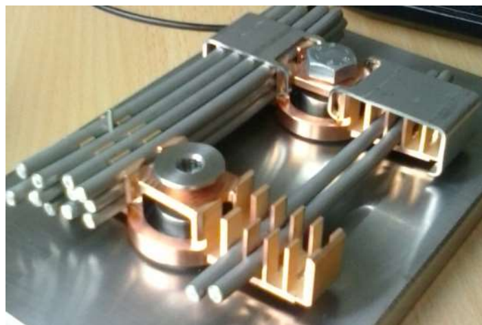
Figure 1. Prototypes of ITER cable looms ready to be tested.
